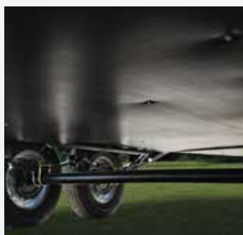
Heated and Enclosed Underbelly Prevents waterlines from freezing in cooler temperatures and greatly extends the camping season.
