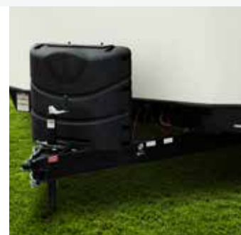
Detachable Hitch Park ready with an easy-to-remove hitch.
