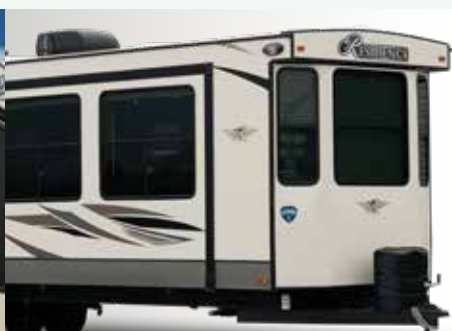
Dual Pane Windows (laminated only) Optional dual pane windows reduce noise and increases the trailer's energy efficiency.
